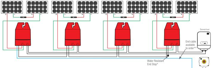
If the array has an odd number of panels, a single panel can be connected directly to the positive (+) and negative (-) panel cables of the BFS.
